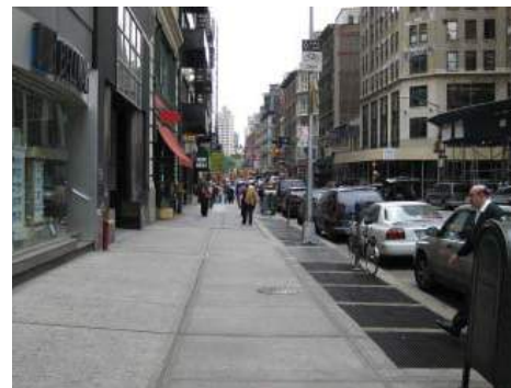
Vaults to building basements and long strips of subway grates will dictate to some extent the placement of streetscape amenities.
